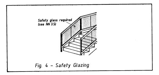
If it is required to locate a window at a distance less than 1 800 mm above the pitch line of the stairs or landing as the case may be, it must be glazed with safety glass (see Figure 5).
