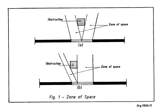
**OO3.3** Any such zone of space shall be limited by parallel planes passing through and extending from the highest and lowest points of such opening and by parallel planes passing through and extending from the points of such opening that are furthest apart in the lateral direction.
